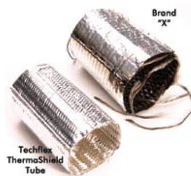
Techflex ThermaShield and a competitor's similar product were placed in the same electrical test oven for one hour at 626°F (330°C). Note the burning and delamination of the fiberglass interior of the Brand "X" product. Even the metallic shroud suffered a degree of burning and brittleness that did not occur on the ThermaShield sample.
